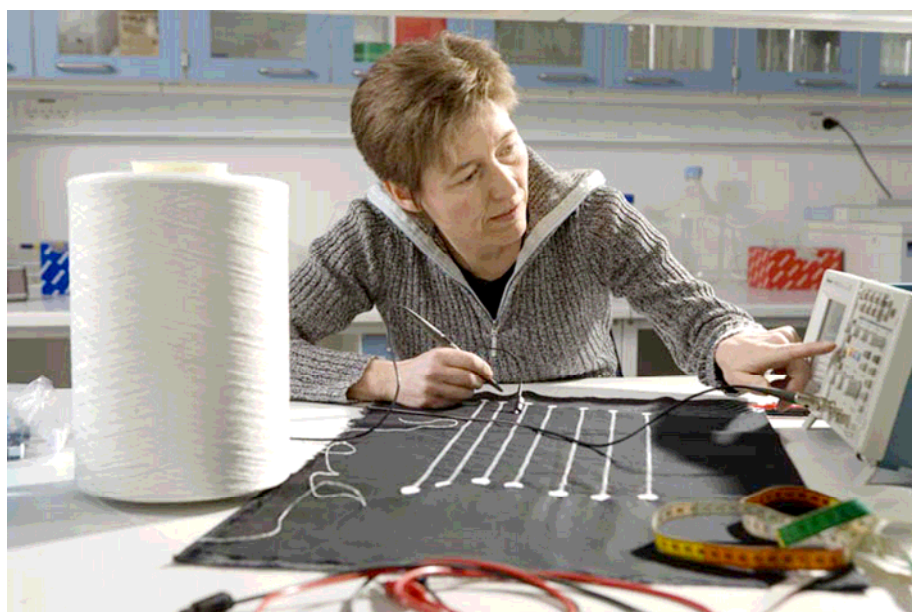
Figure 1: Smart textile development comprises conductive yarns, embroidered sensors and embedded micro-electronics. (Photo: Ohmatex)
