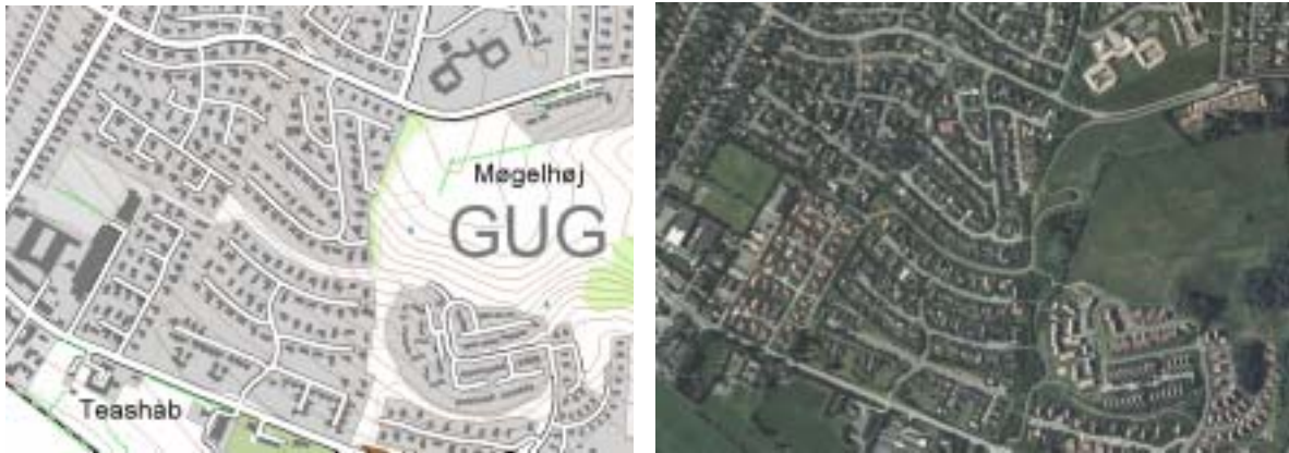
Figure 3. Examples of digital map databases. Left the topographic database TOP10DK produced by the National Survey & Cadastre. Right a colour orthophoto database produced by the private company Kampsax.
