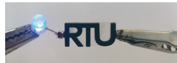
Figure: 3D printed bio-based highly conductive structure with attached LED at 3V
