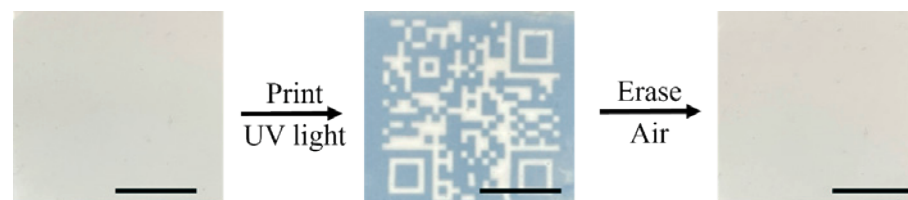
Figure: Photographs of printing and erasing QR code on the photochromic elastomer. Scale bars, 1 mm.
